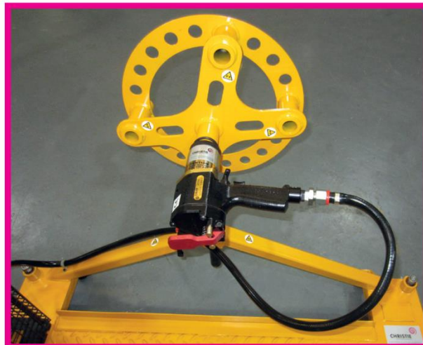
Bus wheel rotation test
