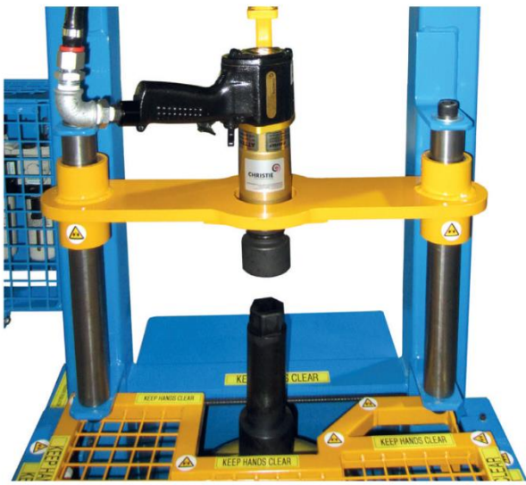
Valve tightening & removal
