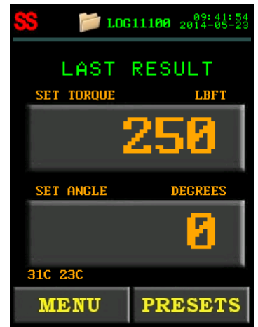
Figure 5.5-3: Passed Last Result With a Smart Socket Not Connected
