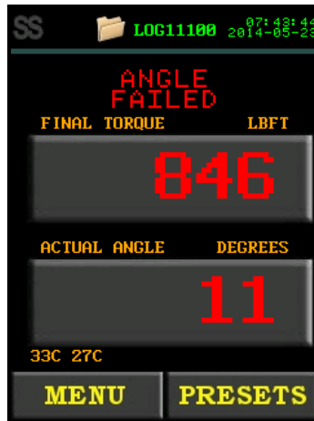
Figure 5.4-5: Failed Torque and Angle Cycle With the Bluetooth Bridge Disabled
