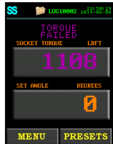
Figure 5.2-2: Failed Torque Cycle
