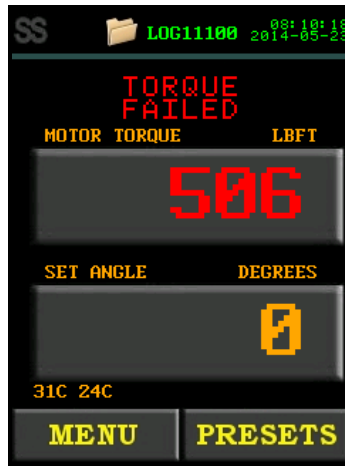
Figure 5.2-4: Failed Torque Cycle With the Bluetooth Bridge Disabled
