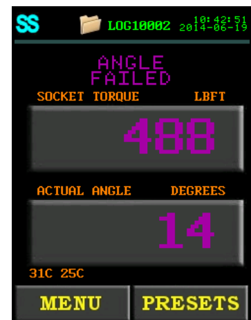
Figure 5.3-3: Failed Angle Cycle
