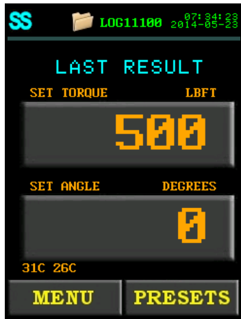
Figure 5.5-1: Passed Last Result With a Smart Socket Connected
