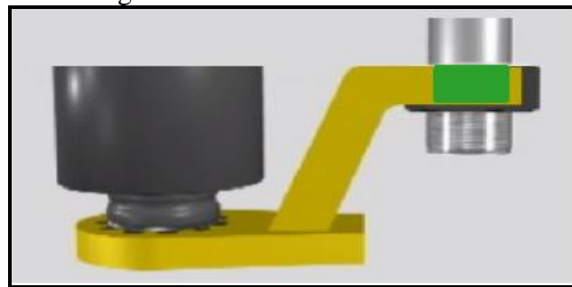
Figure 5.1.4-1: Correct Reaction Point
