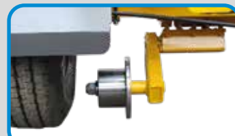
• Retractable Rail Wheel Version for use over inspection pit
