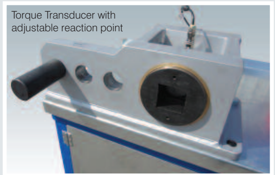
Hand Tool Torque Analyser capable of 1,000 Nm (shown with Calibration Management Readout)
