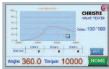
Live graph tracks peak torque
