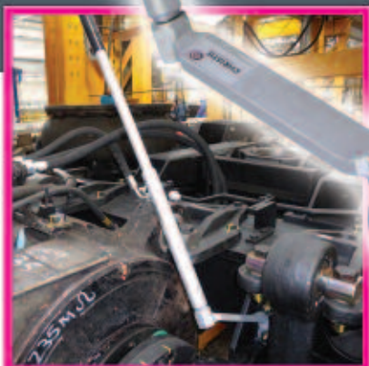
25 mm A/F - 45° Cranked Ring Attachment with Extension Bar
