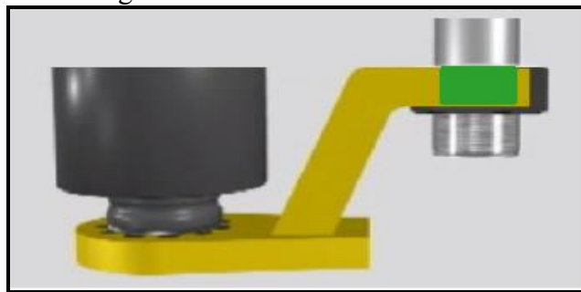
Figure 5.1.4-1: Correct Reaction Point
