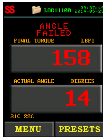
Figure 5.3-7: Failed Angle With a Smart Socket Not Connected
