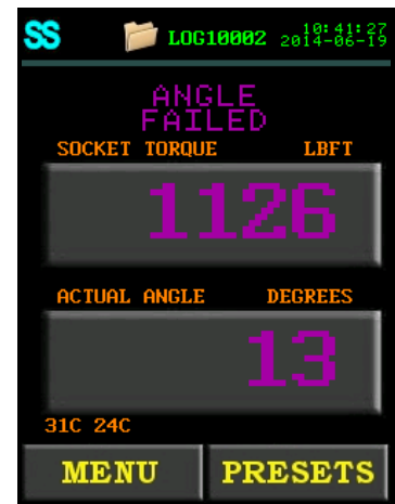
Figure 5.4-3: Failed Torque and Angle Cycle
