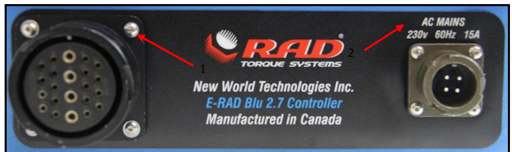
Figure 3.2-1: Controller Cable Connections
