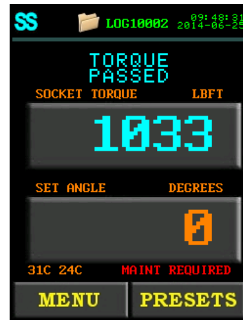
Figure 4.3.17-11: Maintenance Required Warning
