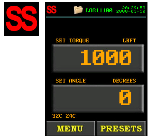
Figure 4.1.1-2: Bridge Found/Enabled. Smart Socket Not Connected
