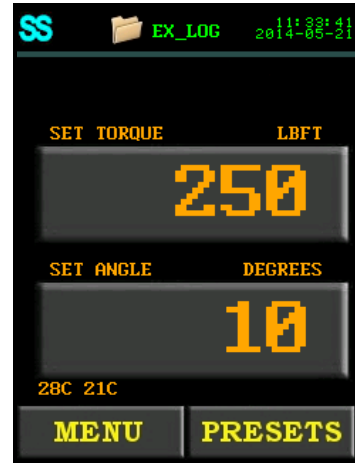
Figure 4.3.3-5: Main Screen with New Data Log Displayed
