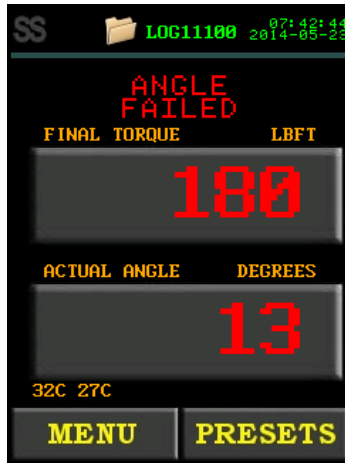
Figure 5.3-5: Failed Angle With the Bluetooth Bridge Disabled
