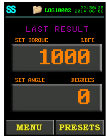
Figure 5.5-5: Failed Last Result With a Smart Socket Connected
