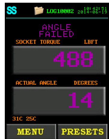
Figure 5.3-3: Failed Angle Cycle
