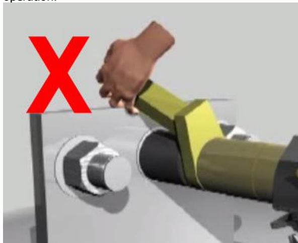
Figure 5.1.1-2: Incorrect Placement of Hand/Body Parts During Operation
