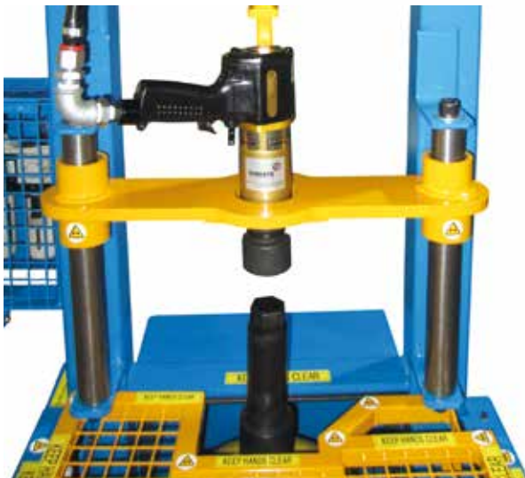
Valve tightening & removal
