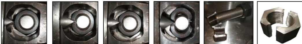
Sequence of photographs showing a typical nut splitting operation. In most cases it is necessary to split the nut on two opposite faces.
